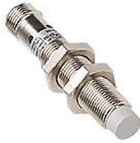
Micro Detectors inductive proximity sensor, tubular, 12mm diameter x 65mm body, nickel-plated brass housing, PNP, N.O. output, 8mm sensing distance, non-flush, 2 kHz switching frequency, IP67, 4-pin M12 quick-disconnect.
